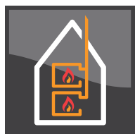
Decentralized multiple fireplaces connected to same chimney
